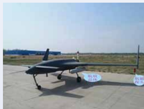
CH-3 UAV-based Airborne Geophysical Prospecting (airborne magnetic/airborne radioactive) Integrated Station “航放晶体” in the picture stands for Crystal for airborne radioactive survey and “航磁探头” for Sonde for airborne magnetic survey
