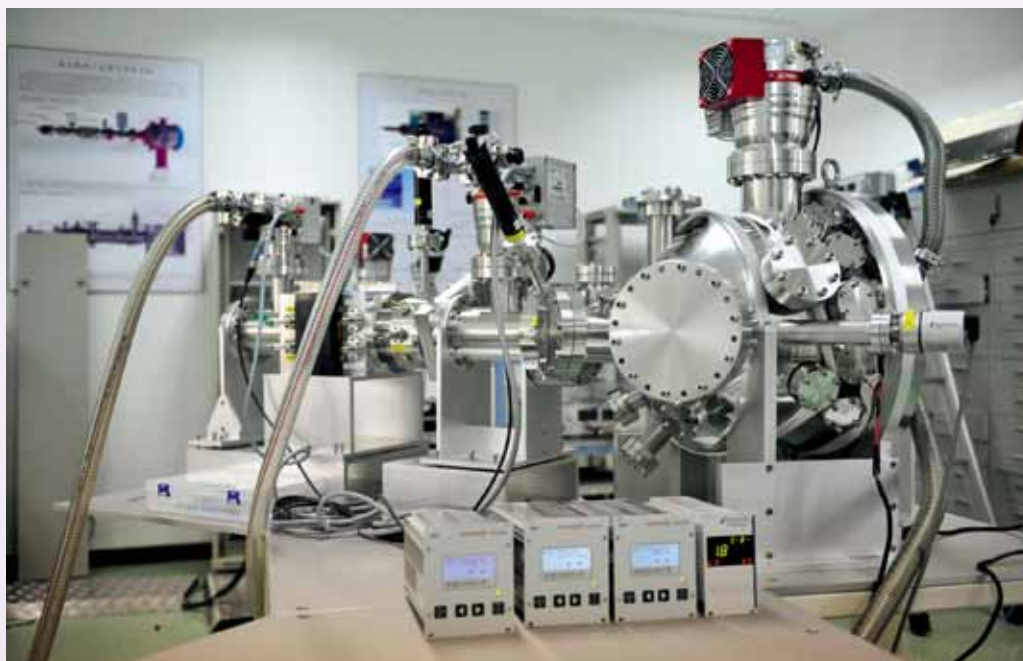
The main chamber of TOF-SIMS-REE
