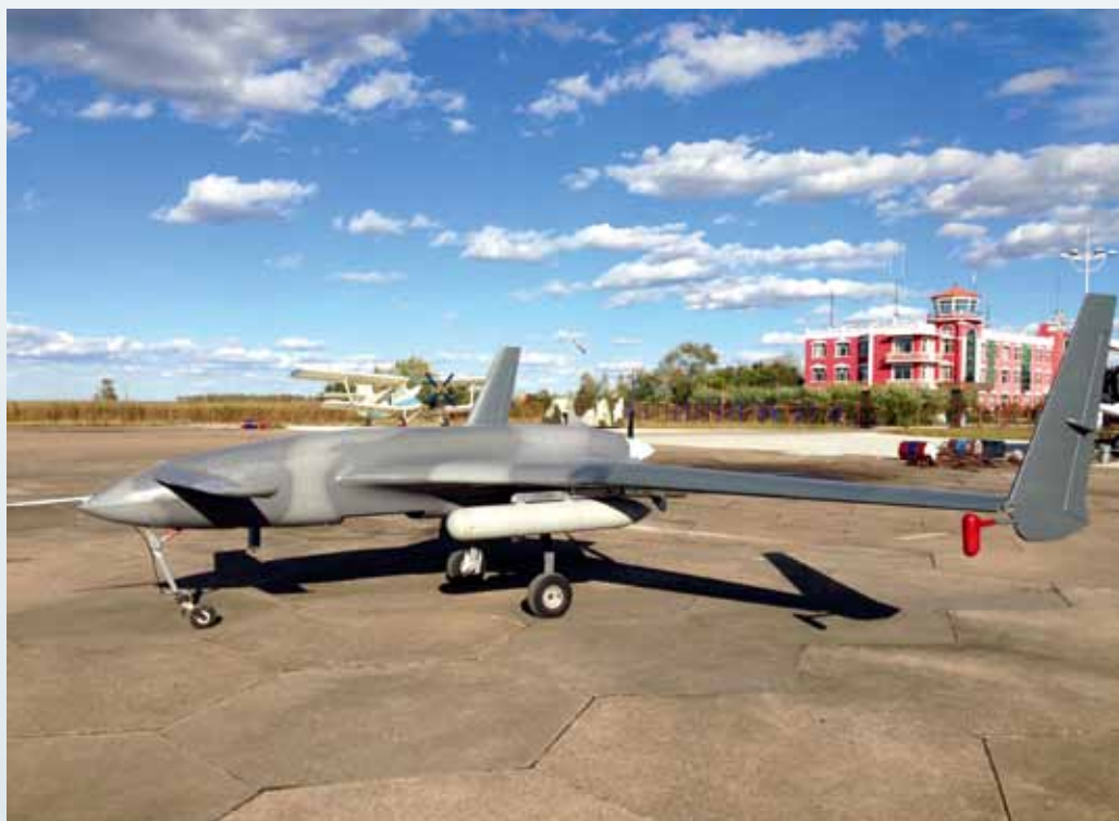
A prototype UAV airborne magnetic/radioactive integrated survey system
