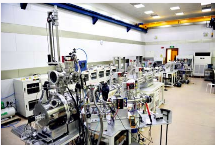
Two TOF-SIMS developed by the technical team of the Centre ( assemblage was completed and testing is in progress)
