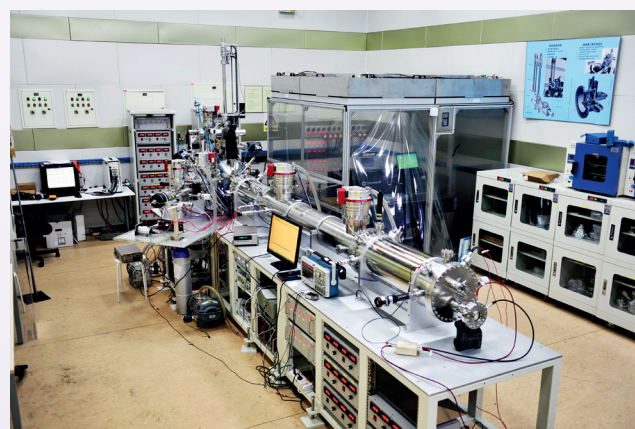
Two units of TOF-SIMS developed by the technical team of the Centre (assemblage was completed and testing is in progress)
